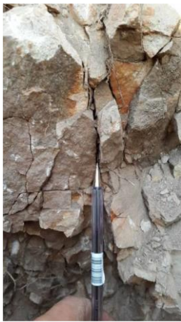
Figure 9 Highly fractured and jointed quartzitic sandstone (PTP 1)
