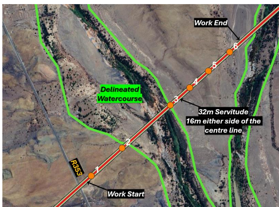
Figure 23. Annotated satellite image of the Leeu Gamka site indicating the extent of maintenance actions, location of pylons to be maintained, main access road and Eskom servitude. All shown in relation to the delineated watercourse.
