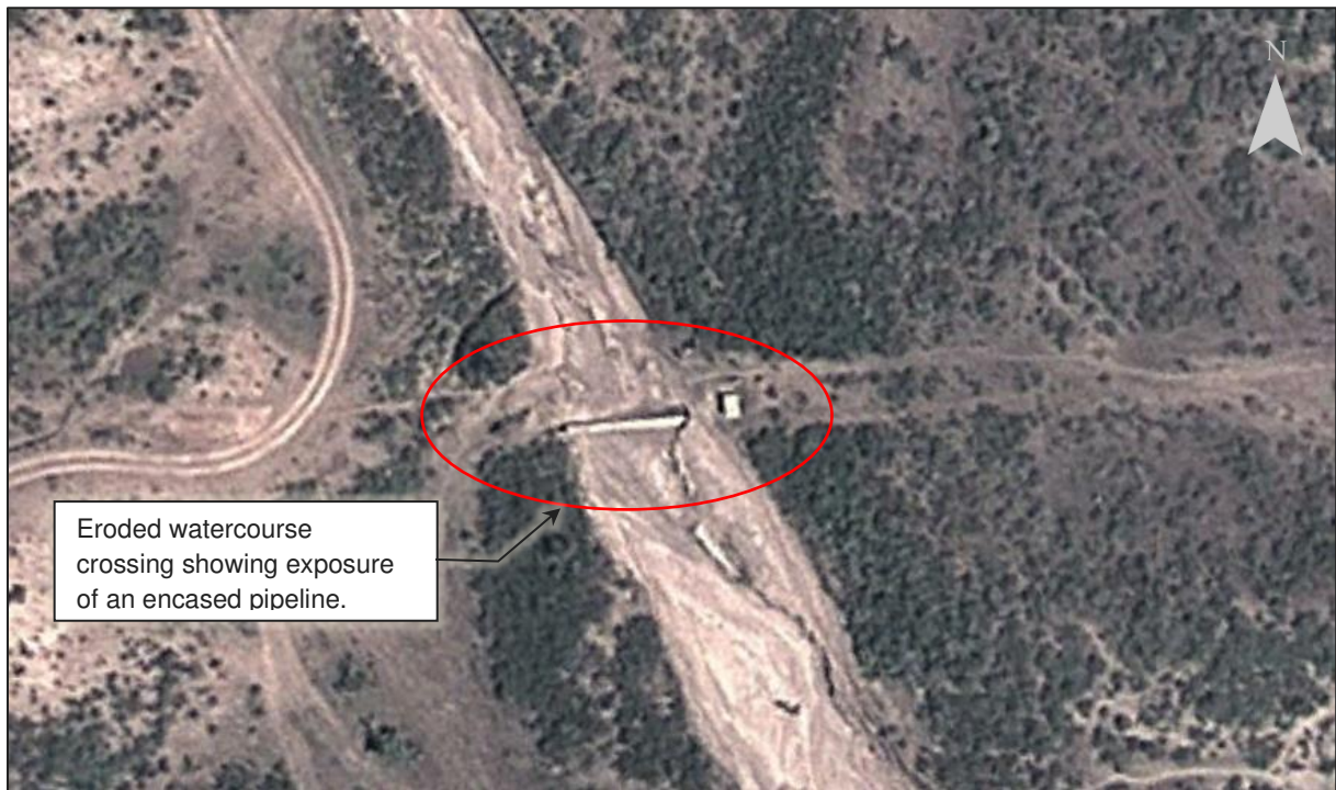
Figure 2-15: Underground pipeline crossing (December 2012), showing the exposed encasement
