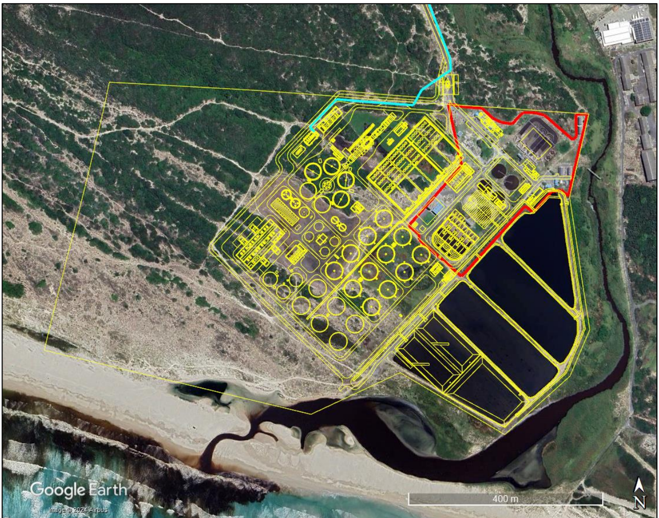
Figure 3: Proposed layout of the expanded Macassar WWTW (yellow). For reference, the red polygon shows the fence line of the existing WWTW. The proposed electric cable is shown in turquoise.
