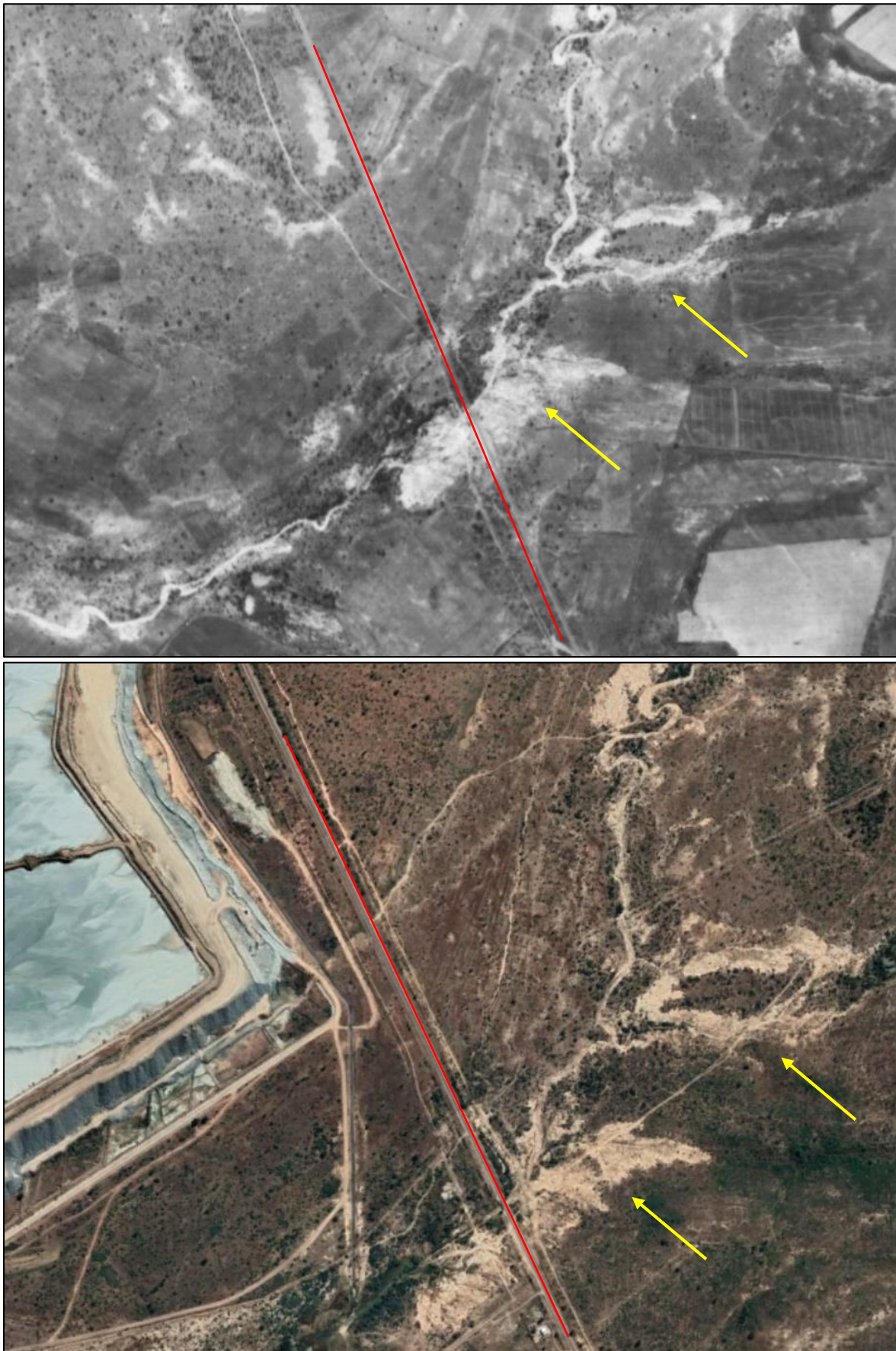
Figure 10: Aerial photographs dated 1967 (top) and current digital satellite imagery dated 2021 (bottom) showing presence of sheet and gully erosion formations in the area. The erosion features (indicted by yellow arrows).
