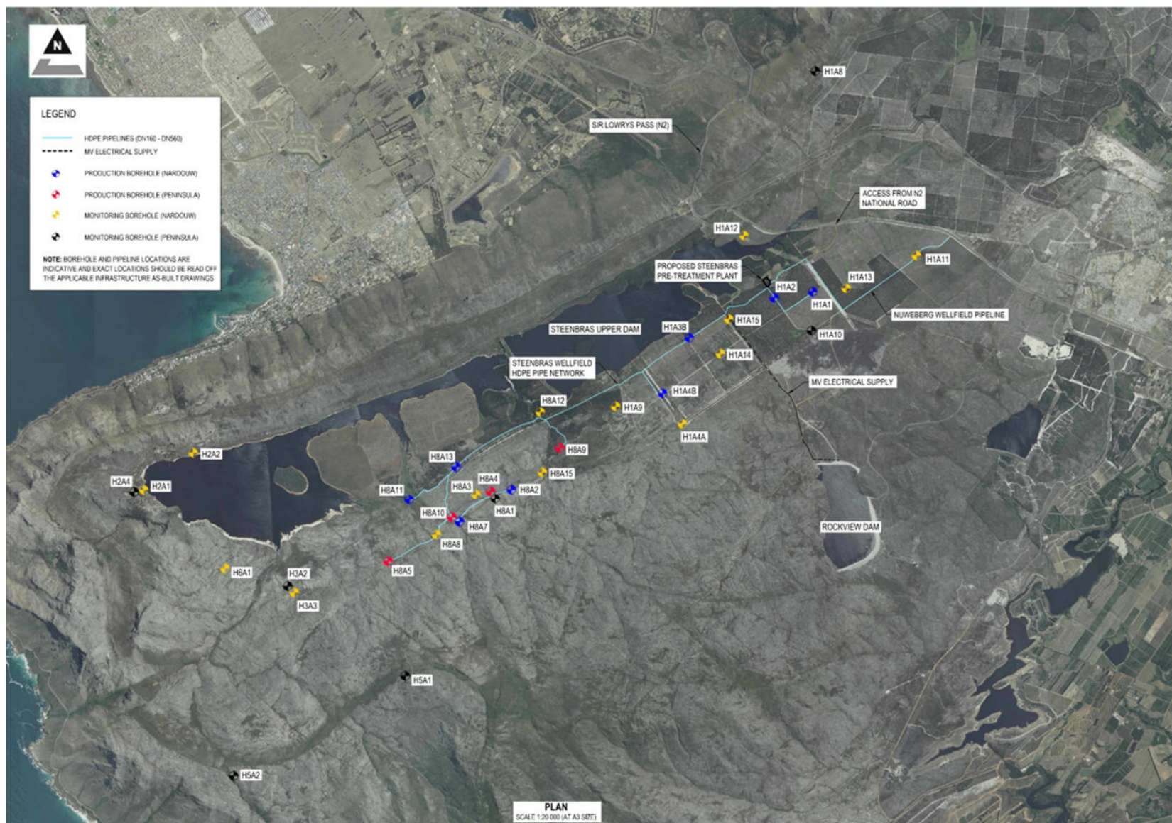
Figure 3: Zoomed out layout of the Steenbras Wellfield to include all monitoring boreholes.
